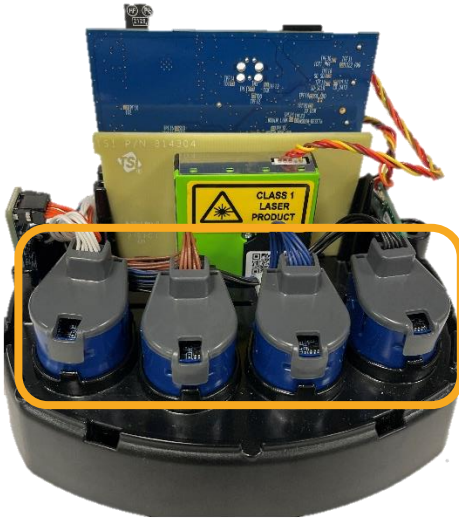
Figure 38: Replace electrochemical sensors
