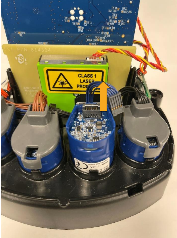
Figure 39: Disconnect sensor cable
