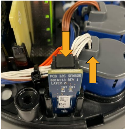
Figure 43: Disconnect sensor cable
