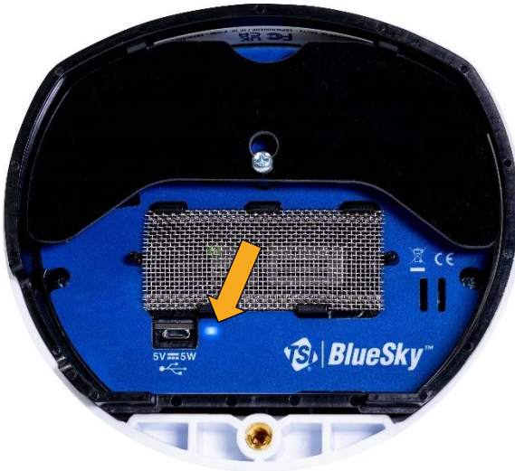
Figure 15: Connections made – LED solid blue
