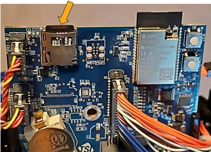
Figure 31: Location of microSD card holder
