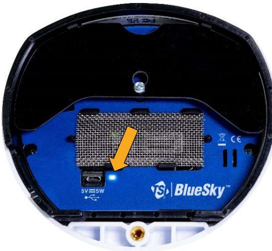
Figure 16: No connection – LED solid white
