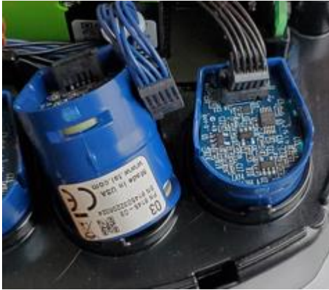
Figure 40: Remove sensor body
