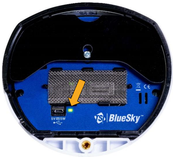
Figure 14: LED pulsing yellow (power cord not shown for clarity)
