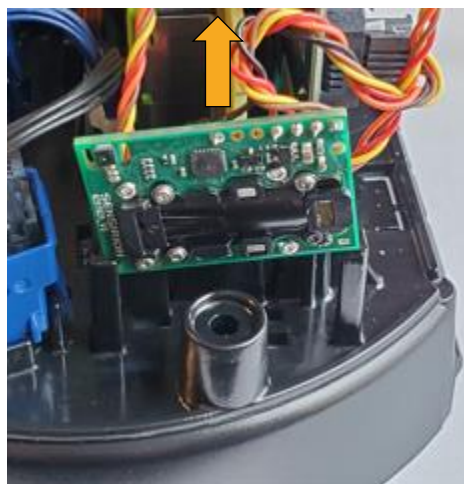
Figure 42: Lift sensor board to remove it
