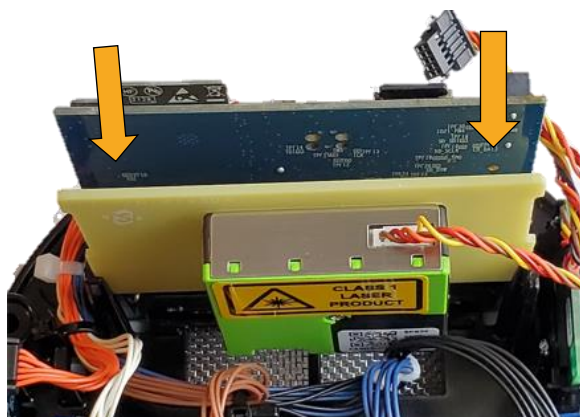
Figure 37: Install new sensor
