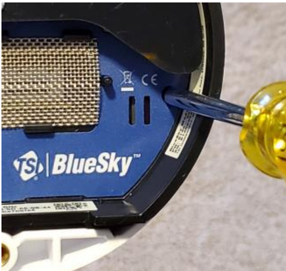
Figure 34: Remove cover screws
