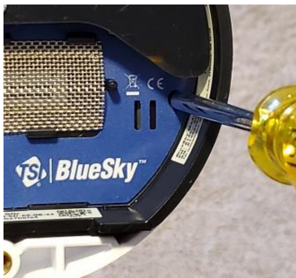
Figure 30: Access microSD card
