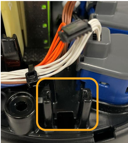
Figure 45: Reconnect cable connector
